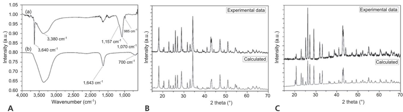
**Figure 4.** **A.** Comparison between the Fourier transformed infrared spectra of Ultracal XS (a) and exogenous material (b) samples. X-ray diffraction plots from **(B)** Ultracal XS and **(C)** exogenous material samples. a.u.: Arbitrary unit. cm: Centimeter.
